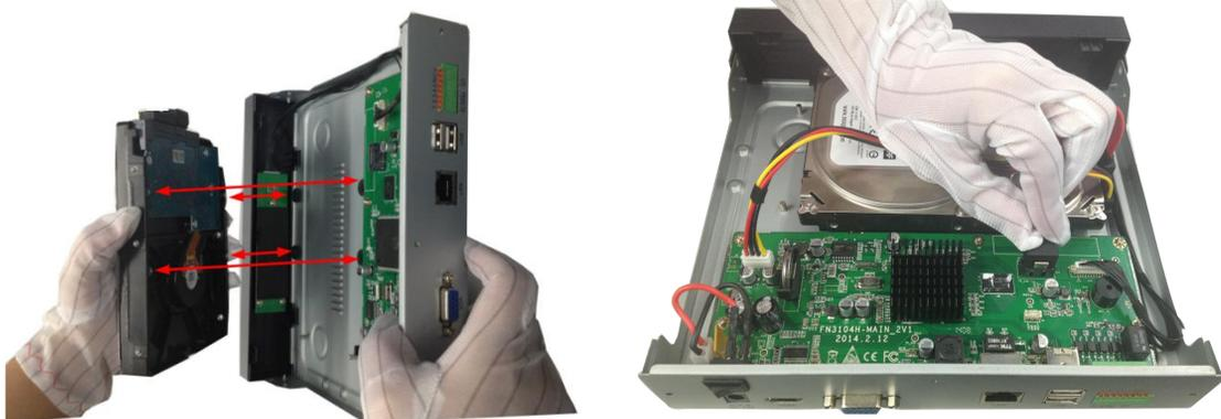
3. Place the HDD on the bottom of the device using the provided screws and then fasten the screws on the bottom to fix the HDD.
