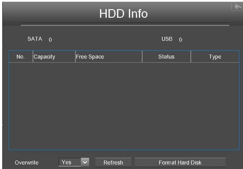
**Overwrite:** When the HDD is full. You can select the whether cover the earliest recording.
